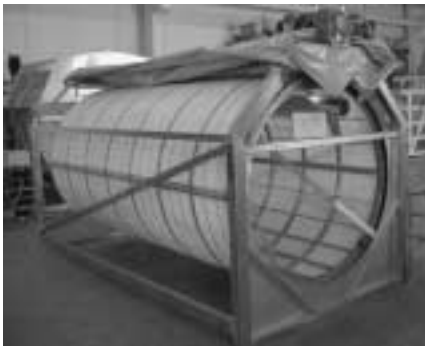
First step is effluent treatment by drumfilter or discfilter
